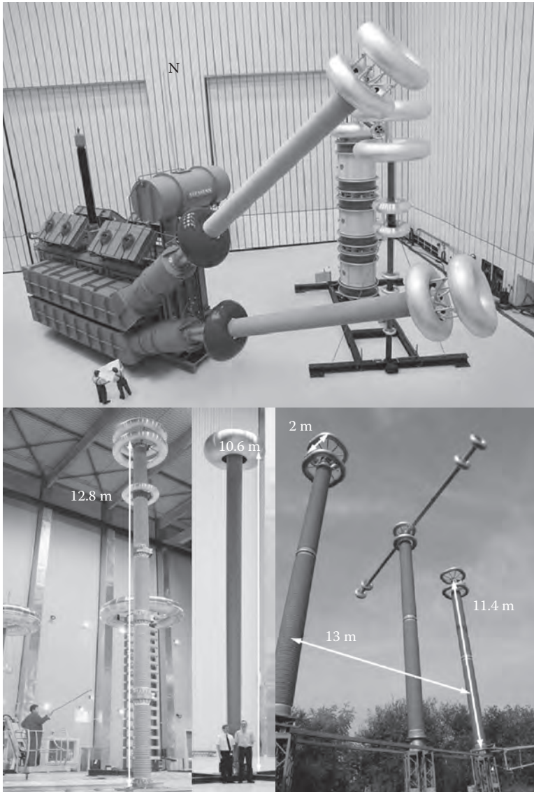
FIGURE 5.17 UHV DC station equipment during testing. Upper part: converter transformer; lower part, from left to right: 800kV DC arrester, DC voltage divider, and DC disconnector.
