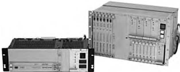
FIGURE 7.2 Remote terminal unit.
