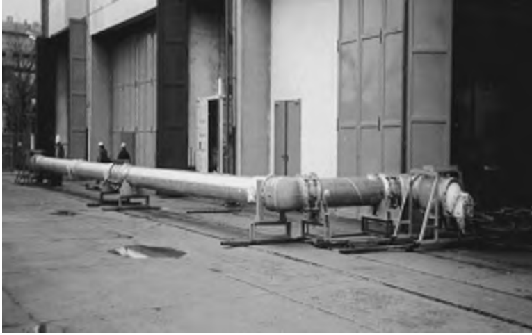
FIGURE 18.11 High-current and internal-arc test setup. (Courtesy of Siemens AG, Erlangen, Germany.)
